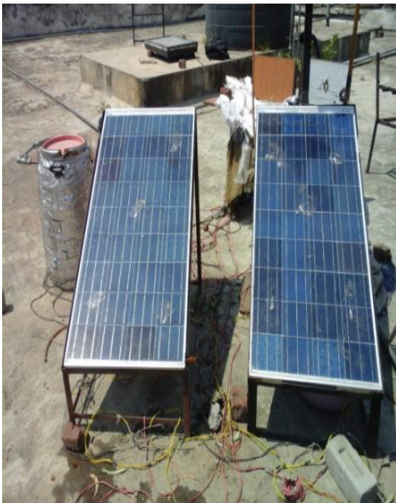
Fig.1: Photographic view of experimental set-up photovoltaic thermal system (left), reference photovoltaic panel (right).
