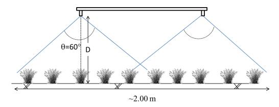
If we take  $\theta = 65^{\circ}$  and D ~ 1.3 m, then theoretical coverage = 1.65 m by single sprayer. So for two sprayer it will be 3.31m.If we consider actual coverage area to be 90 % of
