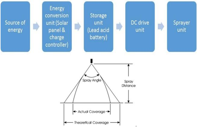
Theoretical coverage of spray nozzle can be calculated using the following equation:
