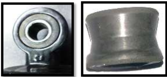
Fig. 7 Test Result for Model 2 (Hardness= 70 shore A)
