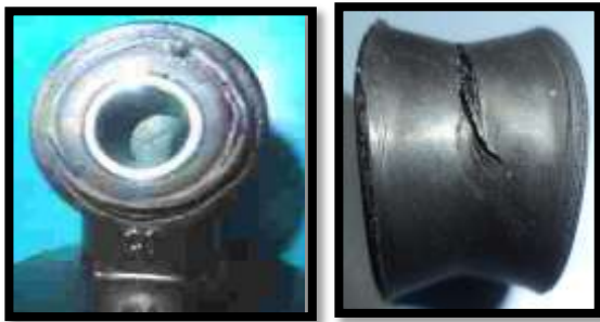
Fig. 6 Test result for Base Model (Hardness= 60 shore A)
