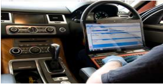
Figure 4.4: PC connected to OBD system
