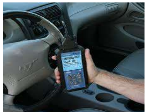
Figure 4.3: Scan tool connected
