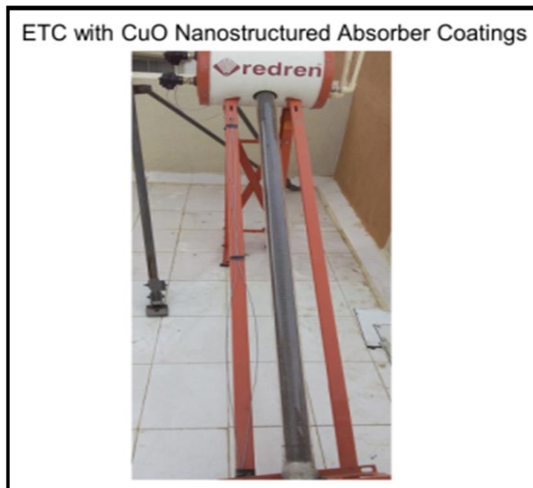
Figure 3: Working setup of Single Evacuated Tube Solar Water Heater Containing Nanofluid
