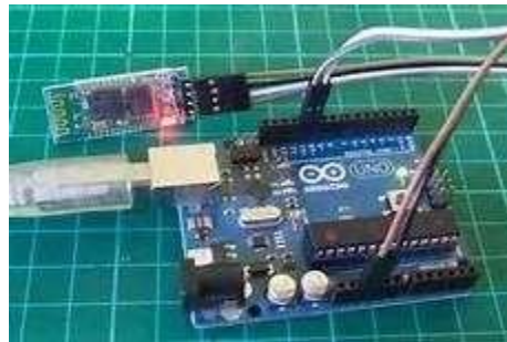
(Figure 2-Arduino board connect with Bluetooth Hc-05)
