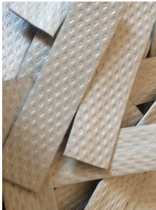
Figure 2: Surface texture and roughness observed on Polypropylene strapping rolls
