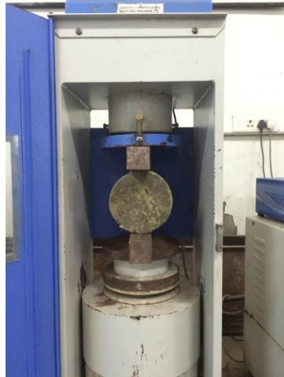
Figure 6: Split tensile test setup
