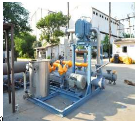
Fig.1. (a) Vacuum Pump in Process (b) Mechanical Vacuum Booster System [3]
