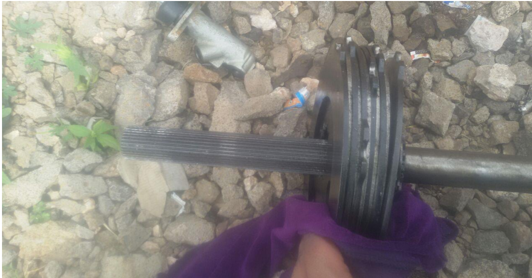
Fig., 5 practically assembly of JCB braking system
