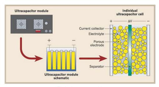
Fig. 1 Ultracapacitor Module
